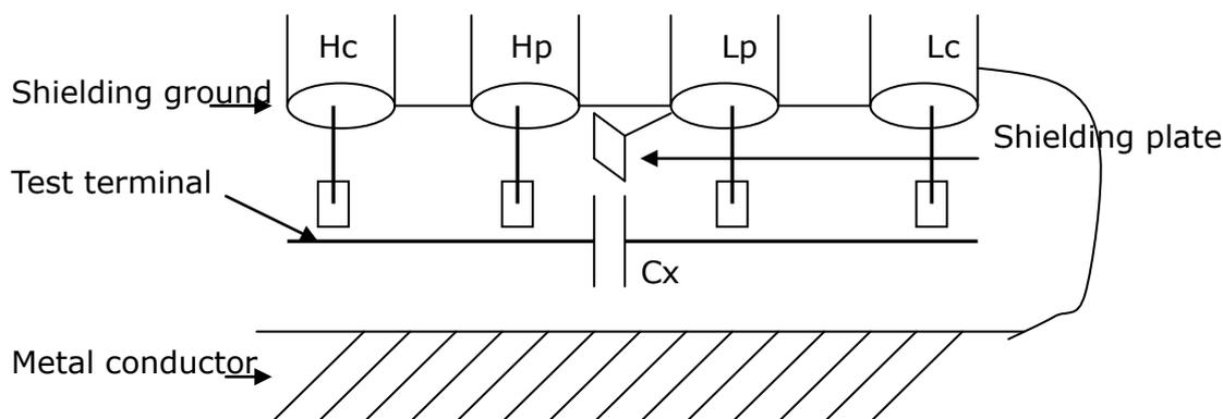
Figure 5-2 Eliminate the influence of stray capacitance
