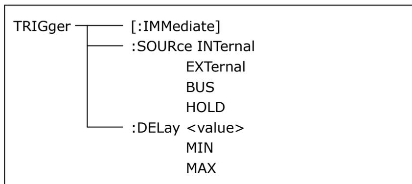
The TRIGger[:IMMEDIATE] command is used to trigger a test.
