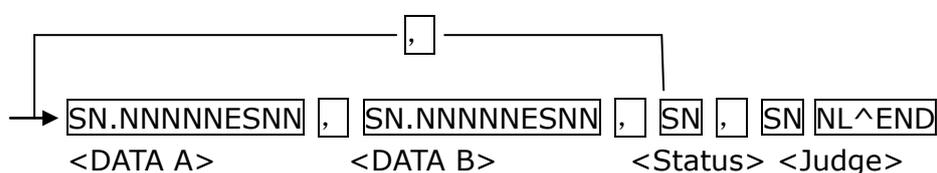
Figure 6 ASCII format 2 (list sweep)
