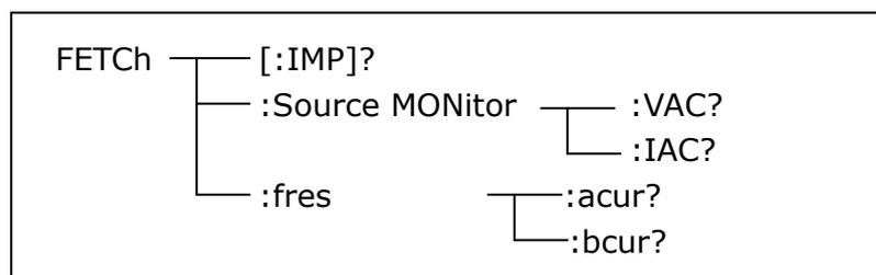
The FETCh[:IMP]? query directs ST2829 to input the last measurement result to the output buffer zone.
